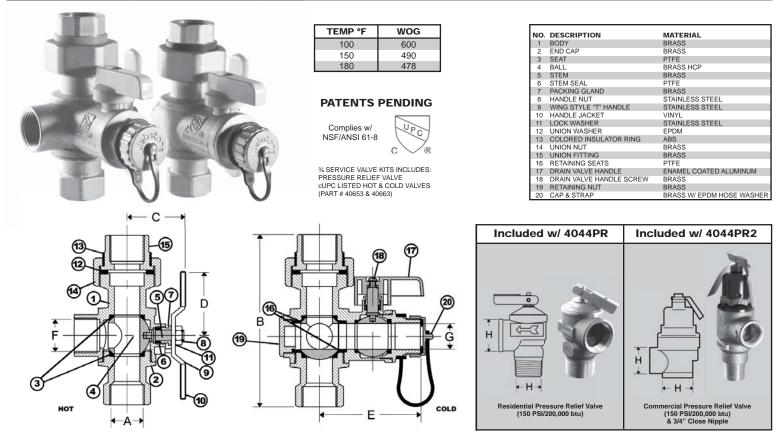
Specifications: Designed for residential, commercial or industrial use with water, oil or gas. This approved Webstone valve features an adjustable packing nut and safety feature that prevents flow from the drain valve when the main valve is in the open position. Threaded ends comply with ANSI B1.20.1. cUPC certification applies to 3/4" models only.
