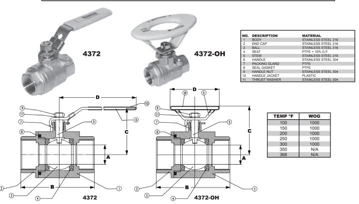
Specifications: Designed for commercial and industrial use with a broad range of fluid handling applications. This approved Webstone valve is actuated by a blowout proof stem and features an adjustable packing nut with locking device. Threaded ends comply with ANSI B1.20.1
