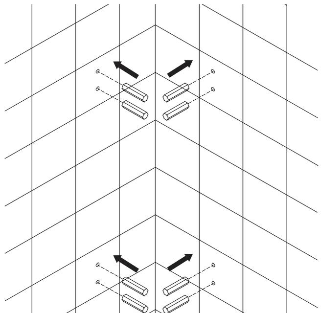
**4** Tighten the screws to the wall with corner brackets
