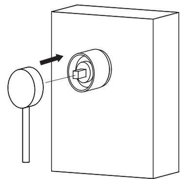
**4** Use allen wrench to fix the HEX screw tightly
