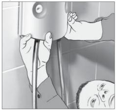
**2** Grip behind the panel, swivel fastening piece into horizontal position.
