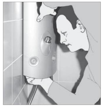
**2** Swivel clamping bracket 90°, tighten wing nut.
