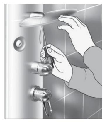
**1** Wall installation + corner installation: Fit glass tray.
