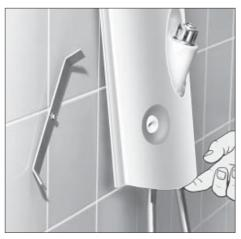
Pull shower panel slightly forwards at the bottom, swivel clamping bracket into position.
