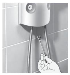
3 Tighten fastening piece nut.
