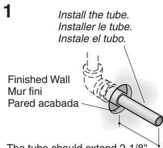
The tube should extend 2-1/8" (5.4 cm) - 3-1/2" (8.9 cm) past the finished wall.
