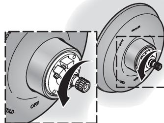
Turn the valve stem counterclockwise to the "OFF" position.
