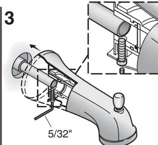
Loosen the setscrew and slide the spout against the wall.
