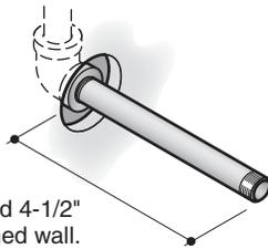
The nipple should extend 4-1/2" (11.4 cm) past the finished wall.
