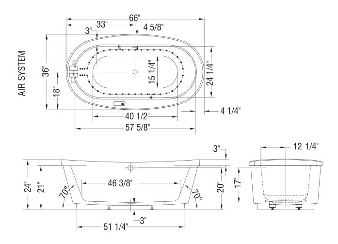
$<sup>\</sup>begin{tabular}{ll} \bullet & ): Indicates airjets positioning \\ ( $\frac{W}{\square} $): Indicates chromatherapy light positioning \\ All dimensions are approximate. Structure measurements \\ must be verified against the unit to ensure proper fit. \\ \end{tabular}$
