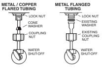
These parts must be used as illustrated to insure water-right connection. Use of existing coupling nut may result in water leakage. Water supply tube or pipe must extend at least 1/2" inside threaded shank of valve (does not apply to flanged tubing).
