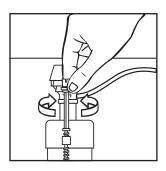
Turn on water supply. Submerge the FLOAT CUP under the water for 30 seconds. Adjust the water to desired level by turning WATER LEVEL ADJUSTMENT ROD and moving FLOAT CUP up or down.
