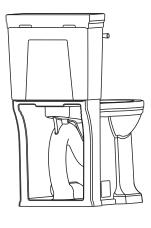
IMPORTANT: Water supply on the wall is required at 3' or 9" from centerline of the toilet (see rough-in). First suggested position is hidden behind the toilet. The geometry of the toilet gives space for this installation. The second suggested position is next to the toilet. Between these two positions, the space for the supply between wall and toilet is limited to 3-1/2". In this case, check your supply and hose dimensions.
