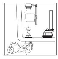
With correct washers in place (see Step 9a), tighten COUPLING NUT 1/4 turn beyond hand tight.
