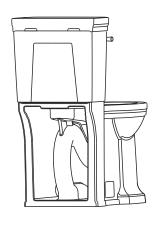
IMPORTANT: Water supply on the wall is required at 3" or 9" from centerline of the toilet (see rough-in). First suggested position is hidden behind the toilet. The geometry of the toilet gives space for this installation. The second suggested position is next to the toilet. Between these two positions, the space for the supply between wall and toilet is limited to 3-1/2". In this case, check your supply and hose dimensions.
