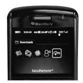
Make sure your Bluetooth<sup>®</sup> is turned on. To pair, your smartphone must be within 80-100 ft. of the SecuRemote<sup>™</sup> device.
