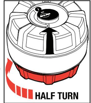
**C** Rotate lower dial half turn to the left till it stops, where the two arrows meet.
