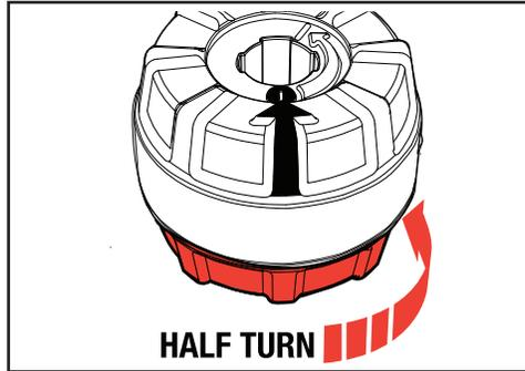
**A** Before you begin, rotate lower dial to the right till it stops to align arrow on upper grip with start point ① on inner dial.
