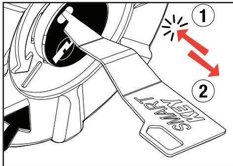
**A** Insert the SmartKey tool into the small hole (next to the keyway) on the cylinder face, and push with force till it goes all the way in, then remove the SmartKey tool.
