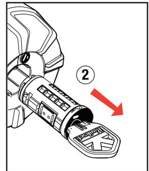
**C** Remove the plug from the reset cradle by gently pulling on the key.
