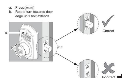
If bolt does not extend, remove lock from door. Follow steps 5-10 to reinstall lock.
