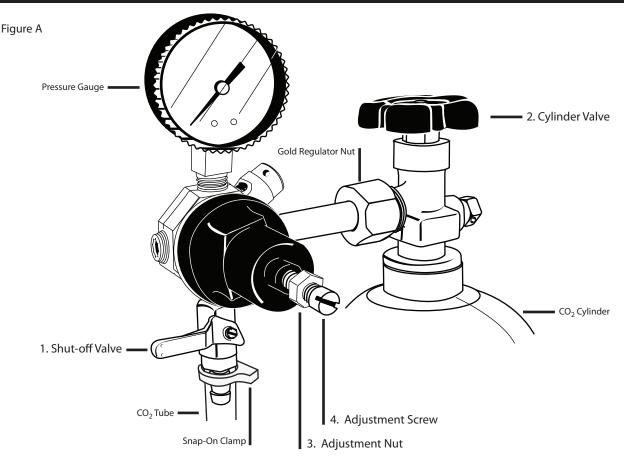
This Regulator Adjustment Guide will help you with those final steps in assuring that your EdgeStar Full Size Kegerator / Keg Beer Cooler provides you with the highest quality tasting beer by walking you step by step through the regulator adjustment process.
