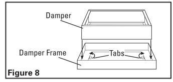
**NOTE:** The damper will only fit into the damper frame one way. If the damper is not fitting flush against the damper frame, turn the damper 90°.
