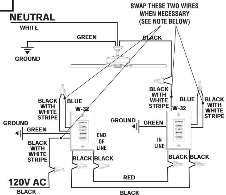
**NOTE:** If wall control operation is reversed (fan switch controls lights and light switch controls fan) turn off the power at the breaker or fuse panel, then swap the two W-32 black/white stripe wires.
