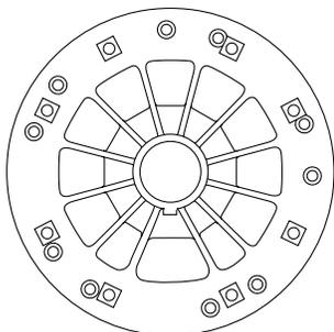
□ = 4-blade mounting hole    ○ = 5-blade mounting hole
