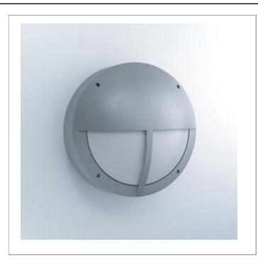
Circular surface mount with domed opal white polycarbonate diffuser with half guard. Exterior grade. Cast aluminum construction with powder coat paint. Unit is complete enclosed.
