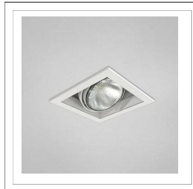
Recessed multi-light fixture series. Designed for remodel applications but also suitable for new construction applications. Adjustable 35° on both axis for aiming in any direction. Cast metal outer trim ring with beveled profile.
