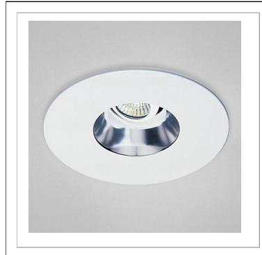
Converts existing 6" housing with medium base to small aperture GU10. Vertically adjustable 0° to 15°; rotates 358°. Complete with medium base to GU10 socket adapter. Compatible with Eurofase 6" PAR housings. Works with most other brands, verification required.
