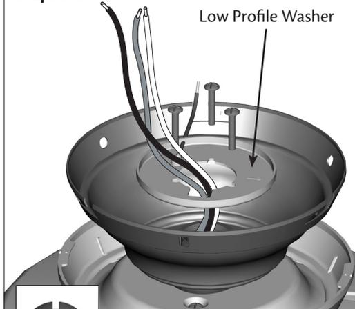
**▲ CAUTION:** The adapter has a special coating on the threads. Do not remove this coating; the coating prevents the downrod from unscrewing. Once assembled, do not remove the downrod.
