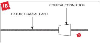
Insert the fixture coaxial cable through the conical connector.
