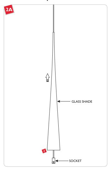
Lift the glass shade up to expose the socket.
