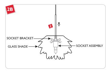
2 Lower the socket assembly into the glass shade to free the socket brackets.
