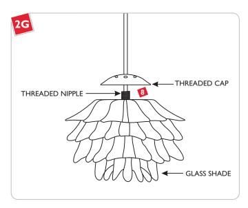
Slide the threaded cap back onto the glass shade and tighten it to the exposed threaded nipple.
