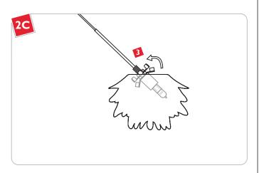
3 Rotate to move the socket assembly from the glass shade.
