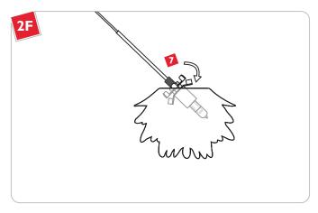
Gently insert the socket assembly into the glass shade at an angle. Rotate so that the socket brackets sit properly around the glass shade collar.
