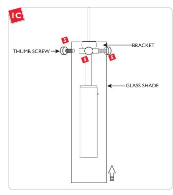
Align the glass shade holes with the bracket holes. Replace and tighten the three thumb screws to secure the glass shade in place. Adjust the thumb screws if the glass is not level.
