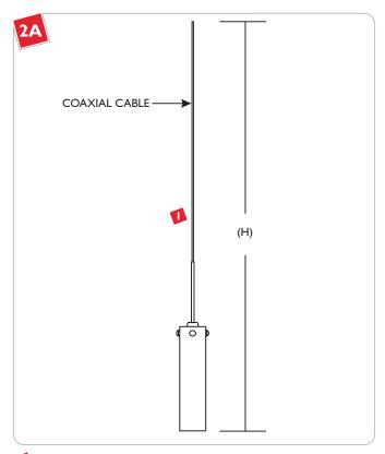
Cut the coaxial cable to the desired length with a sharp cutter. The overall fixture height (H) is measured from bottom of the glass shade to end of the coaxial cable.
