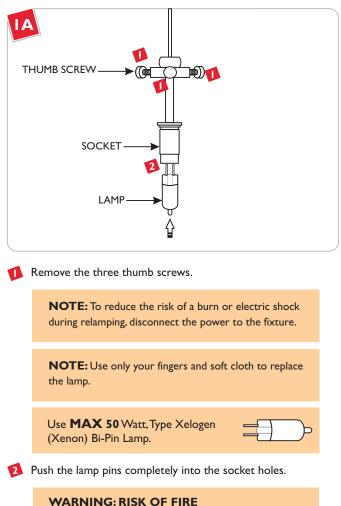
Never replace a Xenon (Xelogen) lamp with a regular Halogen lamp. A regular Halogen lamp requires a protective glass shield.
