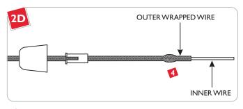
Slide the outer wrapped wire back to expose the inner wire.
