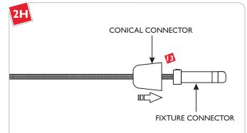
Slide the conical connector over the fixture connector. To install the fixture, refer to the instructions provided with the system.
