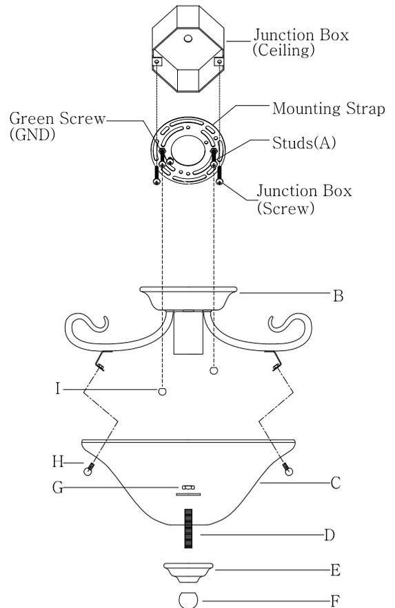
MIN 90°C SUPPLY CONDUCTORS
