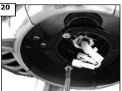
Loosen 2 screws and remove 1 screw and save.
