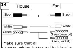
exposed wiring is secured inside wire nuts. Note: Wires from house may vary in color and may not include ground wire. After wiring is conplete, gently push wires into junction box with wire nuts pointing upward. Refer to point 3 of safety tips.
