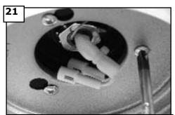
Install the switch housing plate by aligning the 2 screws with the 2 key slot holes on the plate and twist to lock into place. Install the 1 screw removed and tighten the other 2 screws securely.
