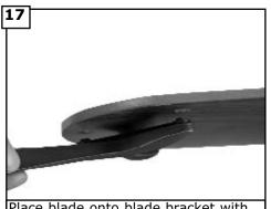
Place blade onto blade bracket with gasket.
