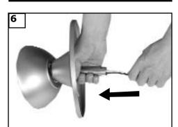
Install canopy and yoke cover over the downrod. Thread wire through downrod with canopy and yoke cover assembled.
