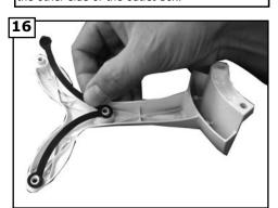
Place the gasket onto the blade bracket as shown above.
