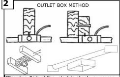
Warning-Risk of fire, electric shock, or personal injury. The fan in this box may be either directly supported from a structural framing member of a building and/or may be mounted to an outlet box marked acceptable for fan support of of 16 kg (35 lbs) or less. Most outlet boxes commonly used for the support of lumminaires may not be acceptable for fan support and may need to be replaced. Consult a qualified electrician if in doubt.
