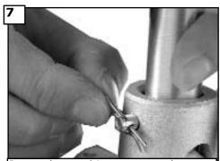
Insert downrod into motor yoke. Next,insert clevis pin through yoke and downrod and secure with cotter pin.
