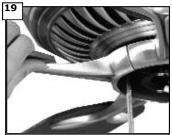
Attach blade assembly to motor using the motor screws and washers provided. Tighten screws securely.
