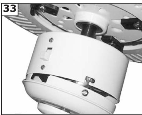
Attach switch cap to fan by lining up 2 slot ear holes and 1 screw hole and twisting cap. Then tighten the 3 screws.
