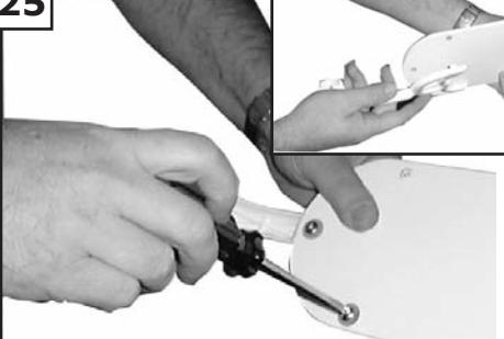
Place blade holders onto blades aligning holes in blade holder with holes in blade. Make sure that the side of the blade you select is facing downward. Install 3 screws and fiber washers to back side of blade as shown. Tighten screws securely. Repeat this process 4 more times until all blades are assembled.
