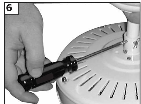
Tighten the 2 Set screws on the Yoke once the downrod is in place. Check motor for shipping stabilizers and remove if present.
