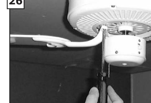
Install blades to motor using the 10 motor screws provided. Tighten screws securely.
