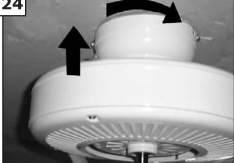
Lift fan to mounting bracket, aligning the "L" shape holes with the screws on the mounting bracket. Turn the fan clockwise to lock in position. Install the 2 canopy mounting bracket screws from the hardware pack and tighten securely.
