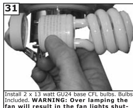
Install 2 x 13 watt GU24 base CFL bulbs. Bulbs Included. **WARNING: Over lamping the fan will result in the fan lights shutting down until the proper wattage of bulbs are installed. Reset the lights by turning off the wall switch, breaker, or by remote. Replace bulbs with the correct wattage bulbs, turn the power on.**
