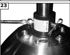
Tighten both yoke set screws to further secure downrod.
