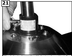
Align holes in downrod and holes in yoke and install cross pin.
