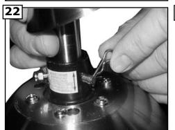
Install cotter pin into cross pin to secure.
