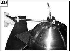
Loosen the 2 yoke screws.
