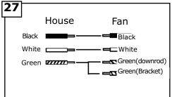
Make wire connections as per above diagram. Connect the white wire from the fan to the White or Neutral wire from the power source. Connect the black wire from the fan to the Black or hot wire from the power source. Connect all Green / Yellow wires from the fan, Downrod and mounting bracket to the Ground wire from the house.
