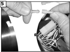
If using the light kit find wires from light and fan body. Plug wires together as follows. Connect blue wire from fan to black wire from light. Connect white wire from fan to white wire from light.
