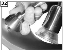
Install the cover of light kit holder tightly over the screw in glass and the slotted arm from fitter. (twist cover counter clockwise)
