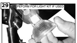
Plug in the 3 light bulbs by aligning the 2 prongs on bulb with holes in socket and then push in and twist the 50 watt bulbs which are GU10 base. Bulbs included. WARNING: Over lamping the fan will result in the fan lights shutting down until the proper wattage of bulbs are installed. Reset the lights by turning off the wall switch, breaker,or by remote. Replace bulbs with the correct wattage bulbs, turn the power on.
