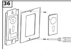
Attach front cover to wall control with screws provided. Snap battery cover in place.
