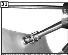
When alligned push screw in glass into the slotted arm from light kit.
