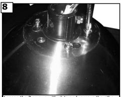
Loosen the 3 screws with slots and remove the other 3 screws. Save the screws.
