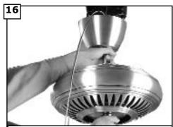
Carefully lift fan assembly onto mounting bracket. Rotate fan so that the notch on the ball engages the ridge in the mounting bracket. This will allow hands-free wiring.
