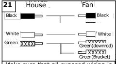
Make sure that all exposed wiring is secured inside wire nuts. Note: Wires from house may vary in color and may not include ground wire. After wiring is conplete, gently push wires into junction box with wire nuts pointing upward. Refer to point 3 of safety tips.
