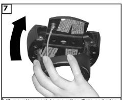
Lift mounting neck to mounting Plate and align
