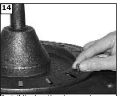
Install the two thumbscrews to secure the yoke cover. Tighten securely.
