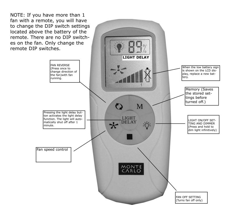
**FAN SPEED** Depress "#1 bar is for highest speed. The #7 bar is for the lowest speed.
