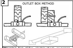
Warning-Risk of fire, electric shock, or personal injury. The fan in this box may be either directly supported from a structural framing member of a building and/or may be mounted to an outlet box marked acceptable for fan support of of 31.8kg (70 lbs) or less. Most outlet boxes commonly used for the support of lumminaires may not be acceptable for fan support and may need to be replaced. Consult a qualified electrician if in doubt.
