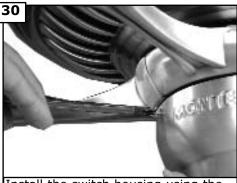
Install the switch housing using the three screws previously removed.
