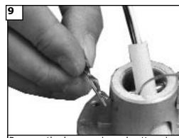
Remove the keeper pin and cotter pin.
