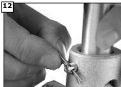
Insert downrod into motor yoke. Next, insert clevis pin through yoke and downrod and secure with cotter pin.
