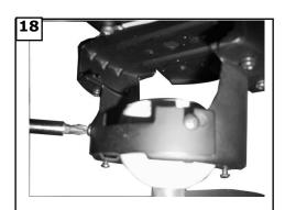
Re-install safety bar removed in step.
