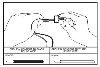
\*Note: When parallel wire is used, the tracer wire is square shaped or ridged and less tracer wire is round in shape or smooth.
