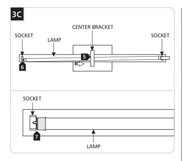
Use MAX 24 WATT type T5 High Output linear fluorescent lamp.
