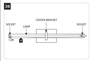
4 Rotate the lamp and carefully slide it out from the sockets and the center bracket.
