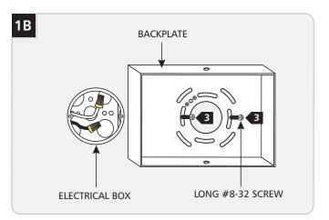
Mount the backplate to the electrical box with two long #8-32 screws.
