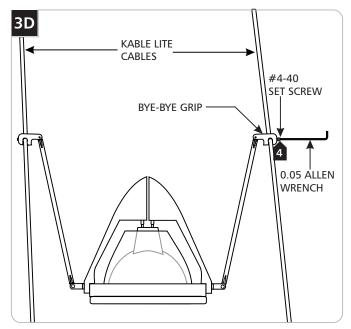
4 Hook each Bye-Bye grip onto one Kable Lite cable and tighten the #4-40 set screw with the 0.05 Allen wrench.
