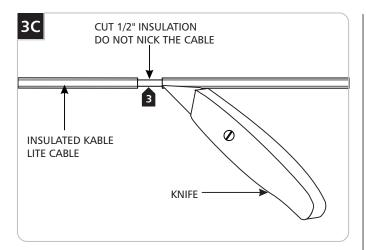
When using Bye-Bye fixture with insulated Kable Lite cables, strip 1/2" of the insulation off with a sharp knife. Make sure not to nick the cable.
