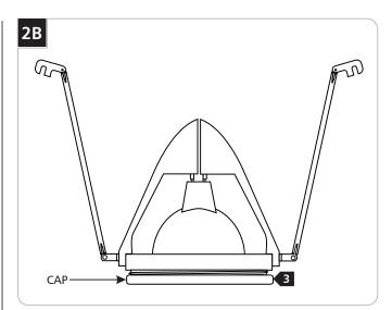
3 Screw the cap back onto the fixture.
