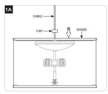
Unscrew the cap from the top of the socket assembly and slide the cap nut off the cable.
