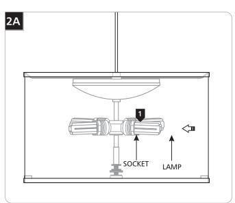
Use **MAX 32** Watt GX24Q-3 Base Triple Tube Compact Fluorescent Lamp with each socket.
