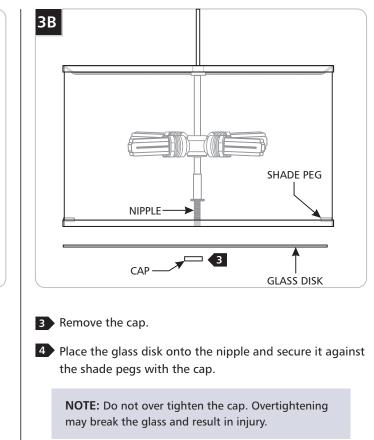
**NOTE:** The lamps can be replaced from the top, without removing the glass disk.
