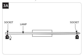
Use MAX 54 Watt type T5 high output linear fluorescent lamp.
