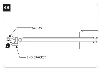
2 Remove the two screws on one end of the fixture and remove the end bracket.
