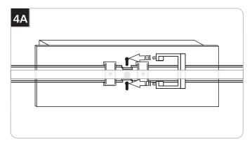
1 Insert the center bracket by aligning the pins to the slotted holes and sliding it into the locked position.
