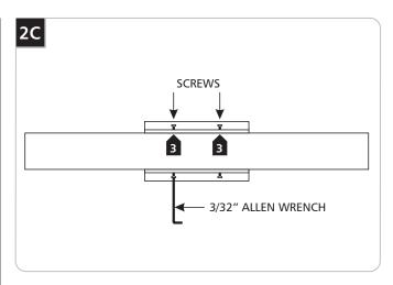
Tighten the four screws on both sides of the backplate with a 3/32" Allen wrench.
