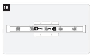
Secure the backplate to the electrical box with the two long #8-32 screws provided.
