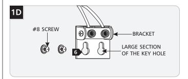
6 Hook the bracket onto the #8 screws through the large section of the key holes.
