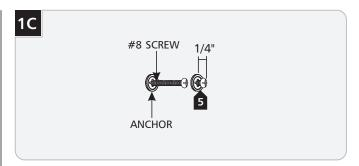
Screw the #8 screws into the anchors. Leave the screws 1/4" exposed.
