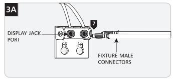
Push the two fixture male connectors all the way into the Display Jack ports.
