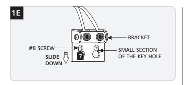
Slide the bracket down so that the small section of the key holes cover the #8 screws. Tighten the #8 screws.
