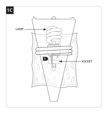
**CAUTION:** To reduce the risk of a burn or electric shock during relamping, disconnect the power to the fixture by turning the wall switch off.
