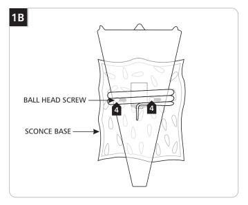
4 Line the sconce base holes with the electrical box holes and secure the plate with two ball head screws.
