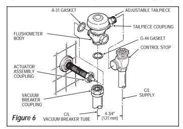
wrench to secure all couplings. This will eliminate damage to chrome or special finish that normally occurs when slip-joint pliers, pipe wrenches or other "toothed" tools are used.
