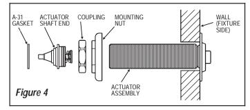
Actuator assembly. Hand tighten Mounting Nut to wall. Securely tighten Actuator Shaft End to Actuator assembly.
