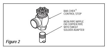
installation of Control Stop on either the left or right side of the valve (refer to Figure 6).
