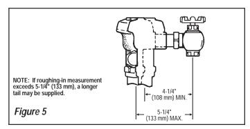
job. Maximum adjustment is 1/2" (13 mm) IN or 1/2" (13 mm) OUT from the standard 4-3/4" (121 mm) (centerline of Flushometer to centerline of Control Stop).
