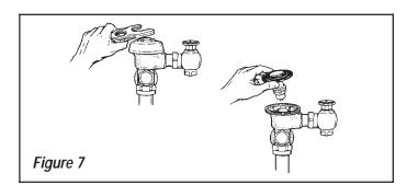
Inside Parts Assembly. Install Flushometer Cover wrench tight. Open Control Stop and activate Flushometer Valve.
