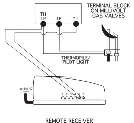
Operation of the remote receiver is similar to that of a thermostat in that both turn the gas valve on and off. A thermostat's input signals are from different temperatures. The remote receiver's input signals are from the transmitter, either manually or thermally.
