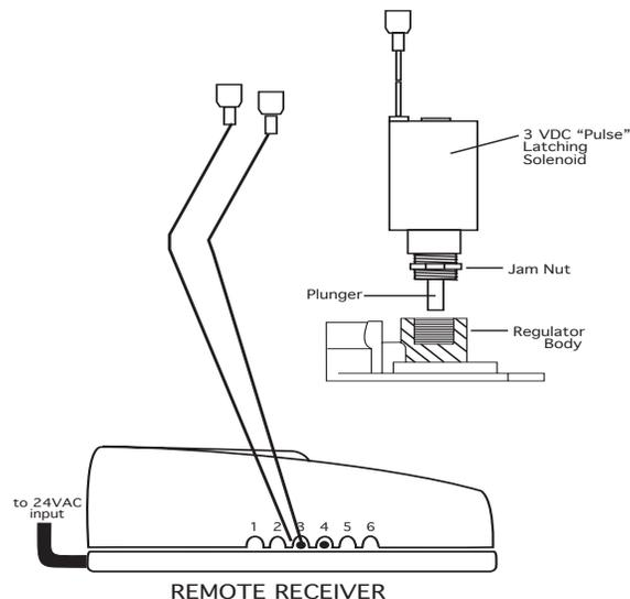
Connect the two ORANGE 18-gauge wires from the remote receiver to the spade terminals on the flame controller. It does not matter which wire goes to the terminal. The input voltage to the flame controller has been changed from 24VAC to 24VDC within the remote.
