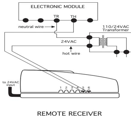
The remote receiver can be connected to a 24 VAC transformer that operates an electronic ignition module, using the same VALVE terminals on the remote receiver to complete the 24 VAC circuit to the electronic ignition module.
