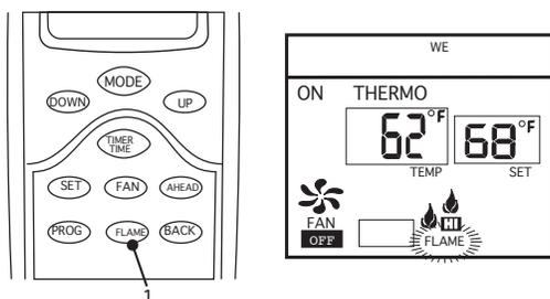
1. Following step 5 above, two flames, words HI FLAME will begin flashing on the LCD screen.
