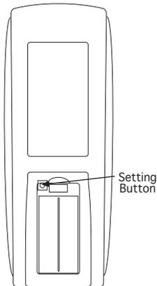
To program settings, first remove the battery cover on the back of the transmitter. If you have not already installed the 2-AAA batteries, this would be a good time to do so. Note the small push button at the upper left side of the battery compartment. This is the button used to perform the initial transmitter programming. You will need to use a paper clip or sharp end of a pencil to depress this button.
