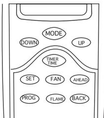
Flashing numbers on the display indicate the system is awaiting user input, such as using the UP and DOWN buttons to program a new setting. If no change is made to flashing digits within 15 seconds, the system will complete the procedure last programmed and reset the display to its normal state.
