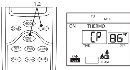
1. To activate the “LOCK-OUT” feature, press and hold the UP and TIMER/TIME buttons, together, for 5 seconds. The letters CP will appear in the TEMP frame on the LCD screen.
