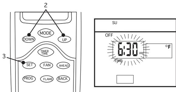
1. Following Step 3 above, the HOUR digits will begin flashing in the TIME frame on the LCD screen.
