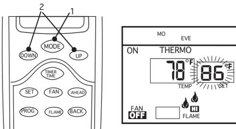
This remote control system can be thermostatically controlled when the transmitter is in the THERMO mode (THERMO must be displayed on the screen).
