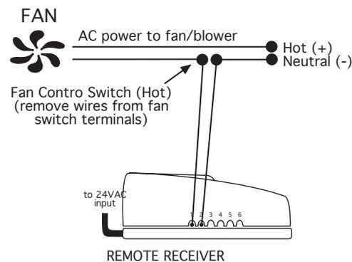
**DO NO CONNECT 110VAC TO WIRES LEADING TO THE REMOTE RECEIVER**
