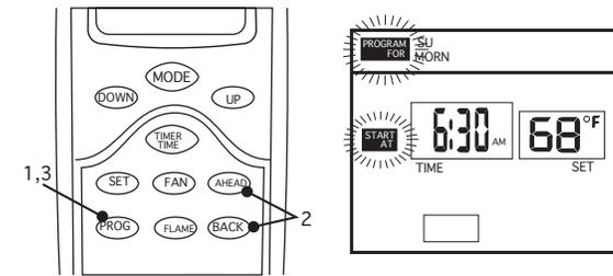
1. Press the PROG button for 4 seconds. The shaded boxes on the LCD screen with the words PROGRAM FOR and START AT will begin to flash. The current DAY, PERIOD, TIME and SET temperature of the BUILT-IN FACTORY PROGRAM will also be displayed.
