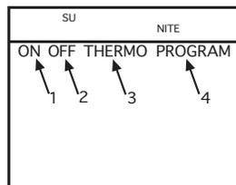
1. **ON** indicates the system is on, either manually or thermostatically.
