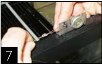
Door roller bracket with metal cable.
