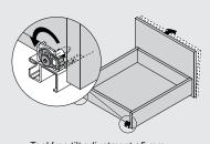
Tool free tilt adjustment +5 mm.
