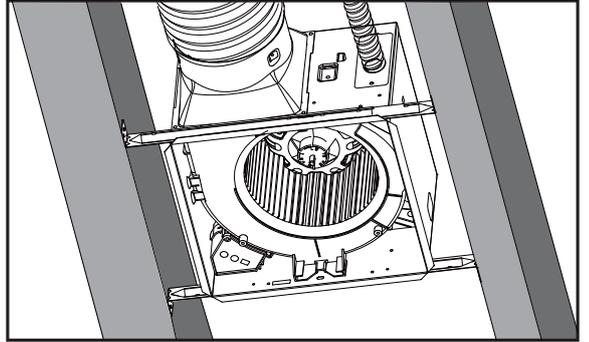
The ducting from this fan to the outside of building has a strong effect on the air flow, noise and energy use of the fan. Use the shortest, straightest duct routing possible for best performance, and avoid installing the fan with smaller ducts than recommended. Insulation around the ducts can reduce energy loss and inhibit mold growth. Fans installed with existing ducts may not achieve their rated air flow.
