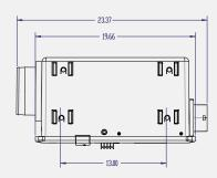
INLET Round collar for 6" dia. duct **OUTLET**Oval collar for 6" dia. duct
