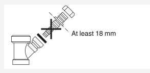
$\overline{\ }$ <sup>2</sup> If the hose is extended, the internal diameter of the coupling must not be less than  $\frac{1}{2}$ ".
