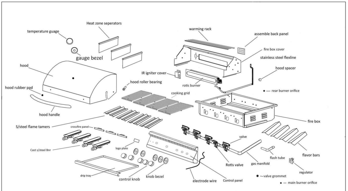
*Note: Add one burner, one flame tamer, one heat separator and one grid for the Blaze 5 Burner.*
