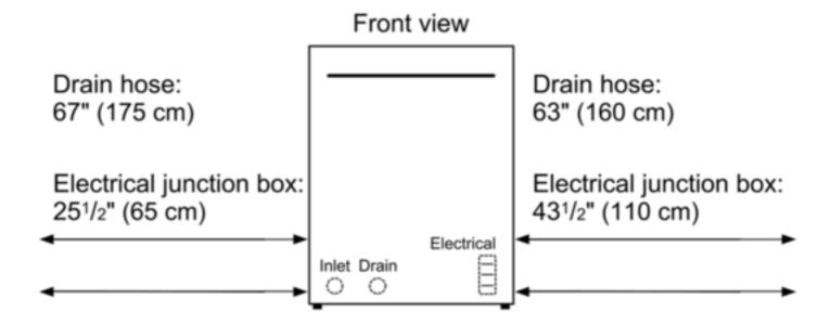
All connections are at the rear of the appliance. Extension for drain hose available as accessory. Power cord for connection to electrical outlet (3-prong plug) available as accessory.
