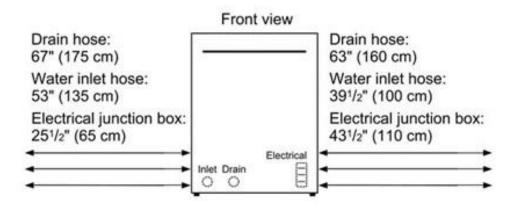
All connections are at the rear of the appliance. Extension for drain hose available as accessory. Power cord for connection to electrical outlet (3-prong plug) available as accessory.
