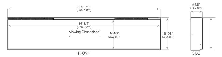
NOTE: The bottom sill needs to be a minimum of 3-1/2" (8.9 cm) deep. The sill can be constructed to support the front of the unit to allow the power supply wires to easily be run behind or flush with the back of the unit and a pass through hole drilled for electrical wire routing.
