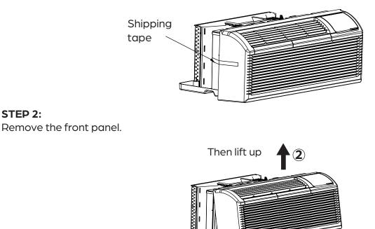
Pull out at the bottom to release it from the tabs.
