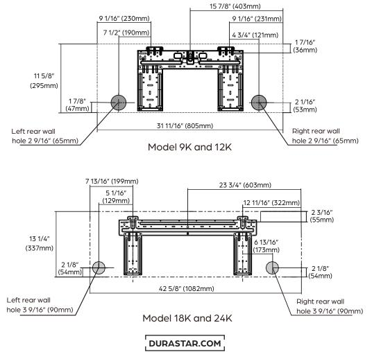
2. Using a 2 1/2" (65mm) core drill for units with a gas side connective pipe less than 5/8" (16mm), or 3 1/2" (90mm) for units with a gas side pipe greater than or equal to 5/8" (16mm), drill a hole in the wall. Make sure that the hole is drilled at a slight downward angle, so that the outdoor end of the hole is lower than the indoor end by about 3/16 – 1/4" (5mm to 7mm). This will ensure proper water drainage.
