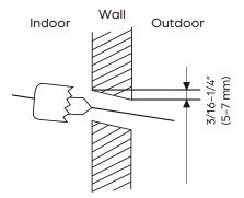
3. Place the protective wall hole sleeve into the hole. This protects pipes and cables from sharp edges and will help seal the opening when you finish the installation process. After the sleeve is inserted through the wall, connect the wall hole cover to the wall sleeve on the outside end. Make sure the cover is flush with the outside wall.
