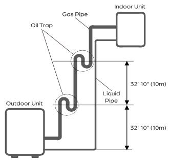
Required distance between oil traps when the indoor unit is installed higher than the outdoor unit.
