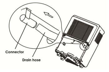
2) Remove the rubber plug from the back of the unit's drain hose outlet, and push the drain hose through.
