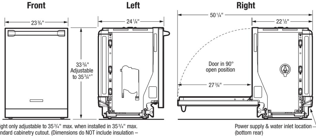
\*Height only adjustable to 35 3/4" max. when installed in 35 3/4" max. standard cabinetry cutout. (Dimensions do NOT include insulation – insulation blanket may be compressed during installation.)
