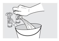
Inspect hose couplings for proper placement of rubber washers. Use hoses from ASSEMBLY HOSE KIT# 5304495002 (not included).
