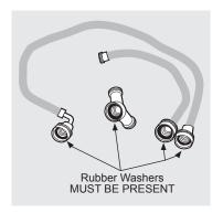
If your installation has room for the COLD water supply to accept the "Y" connector directly, thread the "Y" connector to the COLD water supply and snug it by hand; then tighten it another 2/3 turn with pliers.
