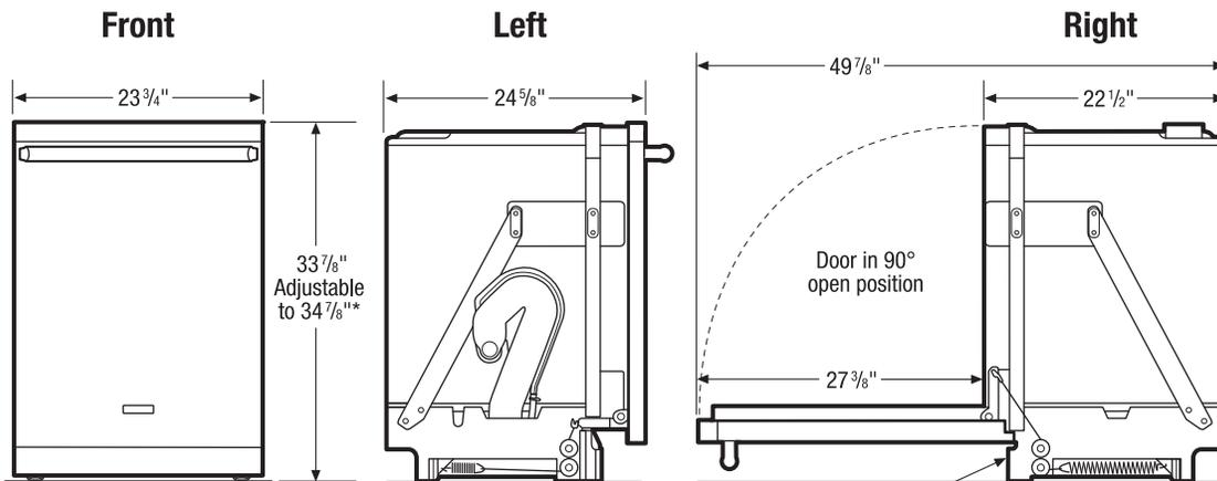
\*Height only adjustable to 34<sup>11</sup>/<sub>16</sub>" max. when installed in 35" max. standard cabinetry cutout
